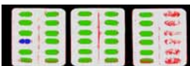
Blister package inspection. Red indicates empty blister, Green indicates normal blister and Blue indicates false product.
